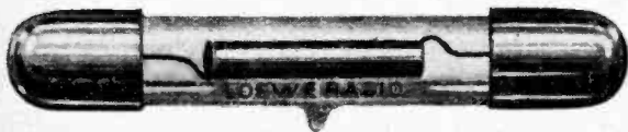
Fig. 2.—Resistance unit consisting of a thin metallic film deposited on a short tube of insulating material
